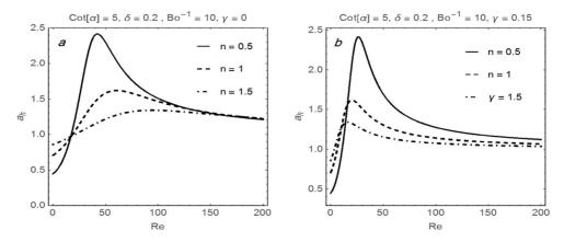
*Fig.* 2. (a, b) Effect of the slip length on the relative amplitude of the free surface up to the first order for different power-law indices n as a function of the Reynolds number Re, at fixed values of the inverse Bond number Bo<sup>-1</sup> = 10, the dimensionless film thickness  $\delta$  = 0.2, and the inclination angle Cot [ $\alpha$ ] = 5.
