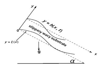
Fig. 1. Sketch of the flow of a power-law fluid over a slippery wavy substrate.
